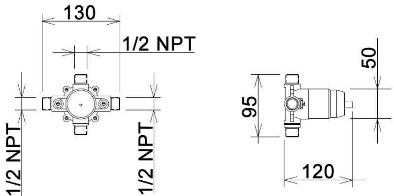
Integrated service stops, filters & back-flow preventers
