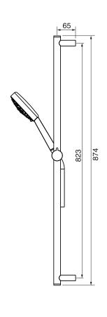
Includes bar, hose and hand shower 3 position spray Easy clean nozzles 2.5 GPM (9.5 L/min.)
