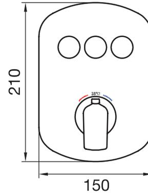
Thermostatic valve with PushGo technology – 3 controls
