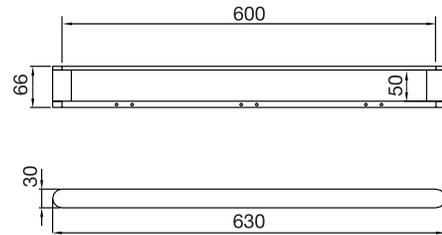
Recommend that brackets are mounted into studs
