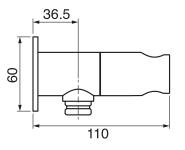
Square metal sprayer with square flange Easy clean nozzles 1/2" male NPT inlet Turn mounting hook for on-off Easy slide installation
