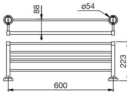
Recommend that brackets are mounted into studs
