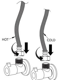
Flush the wall valves to ensure no grit enters the faucet. Now attach the hoses to the wall valves ensuring the hose with RED braid attaches to the hot water outlet.
