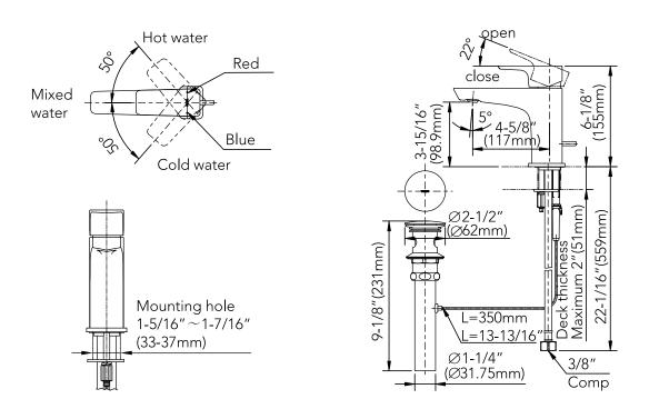
NOTE: The above dimensional unit is inch. The dimension in ( ) is reference mm.
