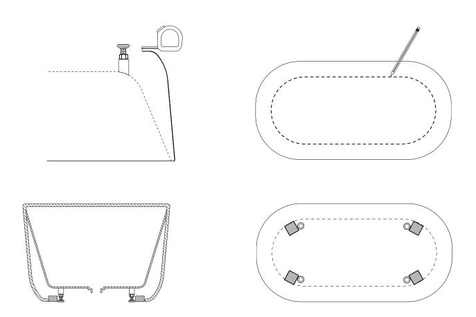
Prepare the plumbing rough-in as required. T.H. Smith bathtubs must be installed using an Island Tub Drain. This simplifies future servicing of the bathtub if required.
