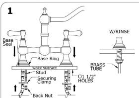
Ensure the mixer is orientated correctly, levers should rotate to point forward. After removing backnuts, place complete faucet through Ø1 3/4" holes at 7 7/8" centers (do not remove unions from body) - product is fitted with straight unions, distance must be exact. Secure mixer with a suitable faucet wrench.
