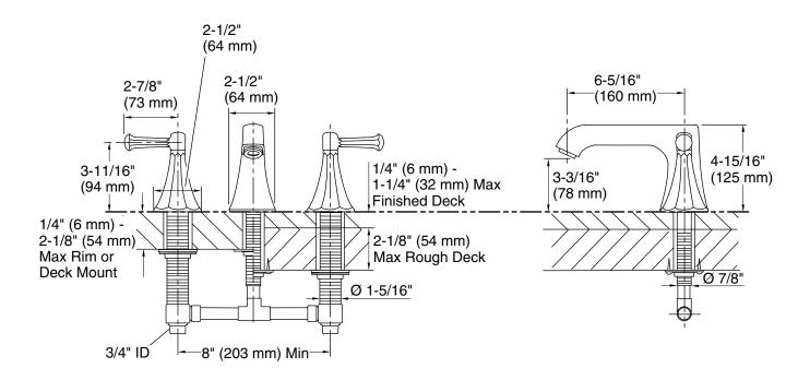
Rim- or Deck-Mount Installation Rough + Finished Deck-Mount Installation
