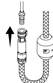
13 Properly tighten the weight on the spray hose, as shown.
