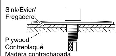
6 Slide on the washers, and thread the ring onto the shank.
