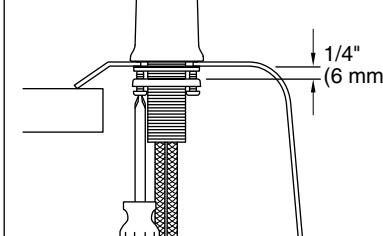
8 Thread each valve escutcheon downward to seal against the countertop. **Do not overtighten!**
