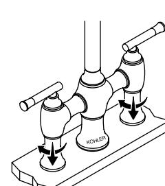
9 Connect and tighten the supply hoses. Turn on the water, and check for leaks.
