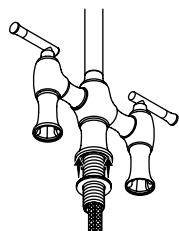
2 With the rubber gaskets facing downward, press a plate into the bottom of each valve escutcheon.
