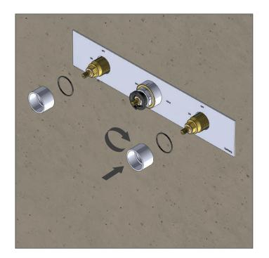
Insert adapter base and tighten
