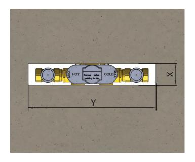
Isenberg's TVH Series valves comes with a black pre-attached mud-guard. This mud-guard is not to be removed or discarded. Its purpose is to guide the installation professional on the proper cut-out dimensions of the drywall.
