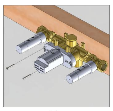
Fix Valve on wooden plank
