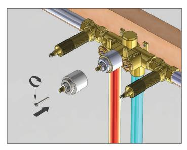
Install thermostatic handle extension and reinsert anti scald temperature ring
