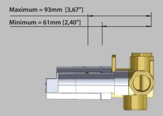
The distance between back of the valve to the finished tile surface should be between 2.40" and 3.67" inches.
