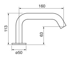
Includes push drain 1.5 GPM (5.7 L/min.)
