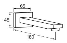
1/2" male NPT inlet Sliding flange Easy slide installation
