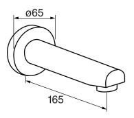
32mm diameter spout 1/2" male NPT inlet Sliding flange Easy slide installation
