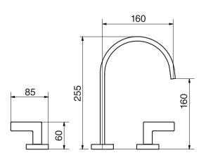
Includes push drain 1.5 GPM (5.7 L/min.)
