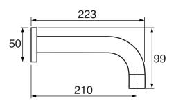
25mm diameter spout 1/2" male NPT inlet Sliding flange
