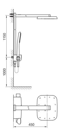
3 control thermostatic mixer with PushGo technology Dual rain head (rain and chute) and hand shower Multiple outlets can be run simultaneously Instant flow when on 2 GPM per outlet (7.5 L/min.)
