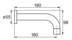
25mm diameter 1/2" male NPT inlet Sliding flange
