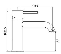
Includes push drain 3/8" flexible supply hose 1.5 GPM (5.7 L/min.)
