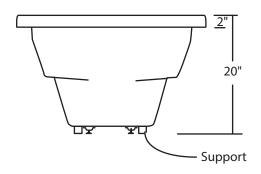
Drain Hole: 2''Overflow:  $2\frac{1}{4}''$ Sizes:  $\pm\frac{1}{4}''$ Diagram not to scale
